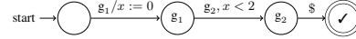
Fig. 13. GEAR. The set W (length 307–1,011,427) is generated by the automatic transmission system model in [16]. The pattern, from \phi_5^{AT} in [16], is for an event in which gear shift occurs too quickly (from the 1st to 2nd).
