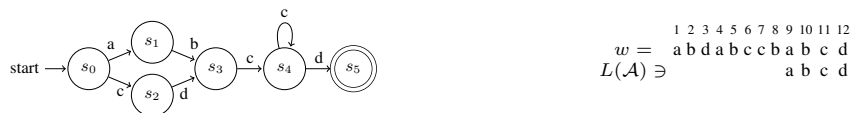
Fig. 4. Pattern matching. For the pattern NFA \mathcal{A} on the left, for which it is easy to see that L(\mathcal{A}) = L(\{ab, cd\}cc^*d) , the output is \{(9, 12)\} as shown on the right.
